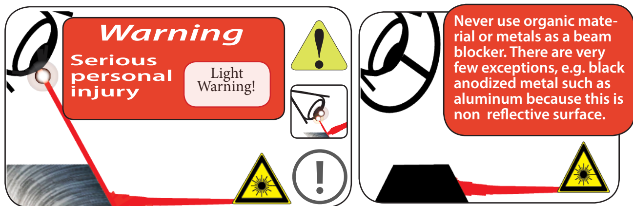
Figure 2-2 Always wear safety glasses or protective goggles with side shields to reduce the risk of damage to the eyes when operating the laser.
